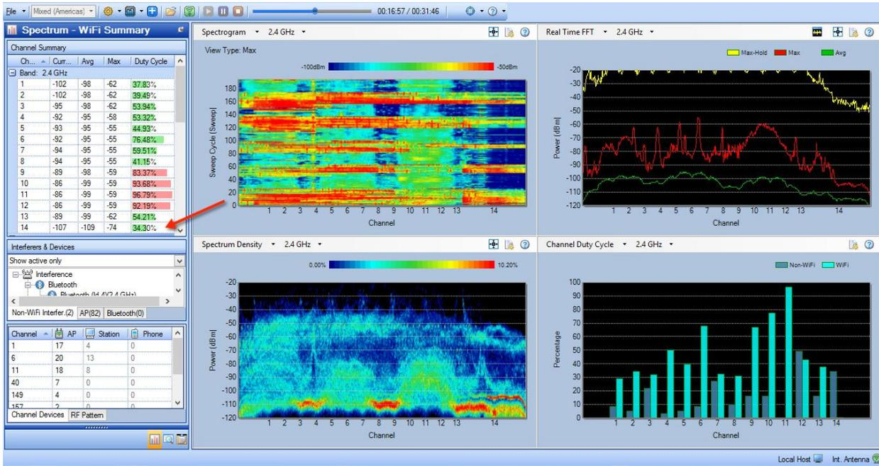
The screenshot above shows the channel utilization (duty cycle) of channels 1-14 in a variety of ways. The most important are the Channel Summary, Spectrogram, and Channel Duty Cycle, so let's zoom in on them, shall we?
